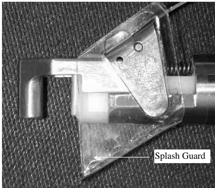
**Figure 2.3 Final Attachment of Splash Guard**
