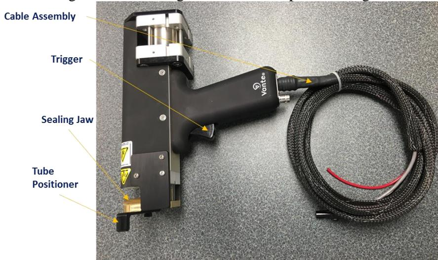
**Figure 2.5 Model 3806MOD (3807MOD is the large size version) midsize tube sealer**
